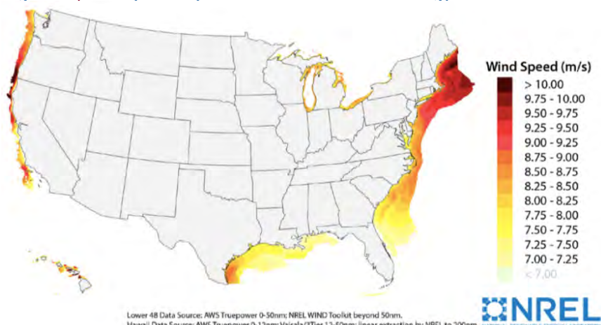
Figure 40 | Wind speed map for the U.S. offshore wind energy technical resource area
